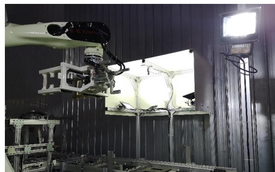
Figure 3. The Physical View of the Appearance Detection Facility
