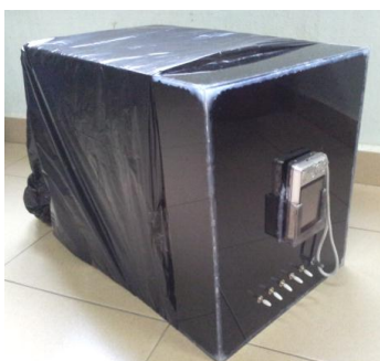
Figure 4. The casing designed to capture face images under the exposure of poor illumination
