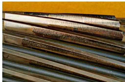
Figure 7. Severe scuffing on the high speed pinion. (courtesy of national renewable energy laboratory)
