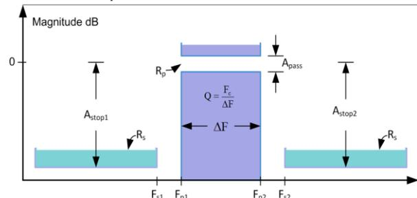
Figure 2. The band pass filter.
