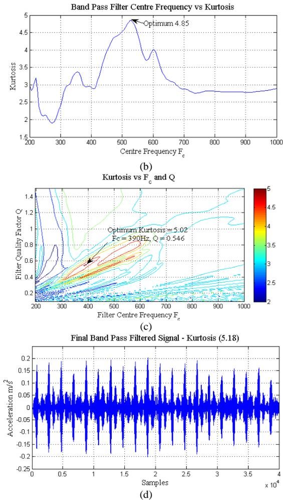
Figure 5. The Chebyshev band pass filter optimized by the PSO.
