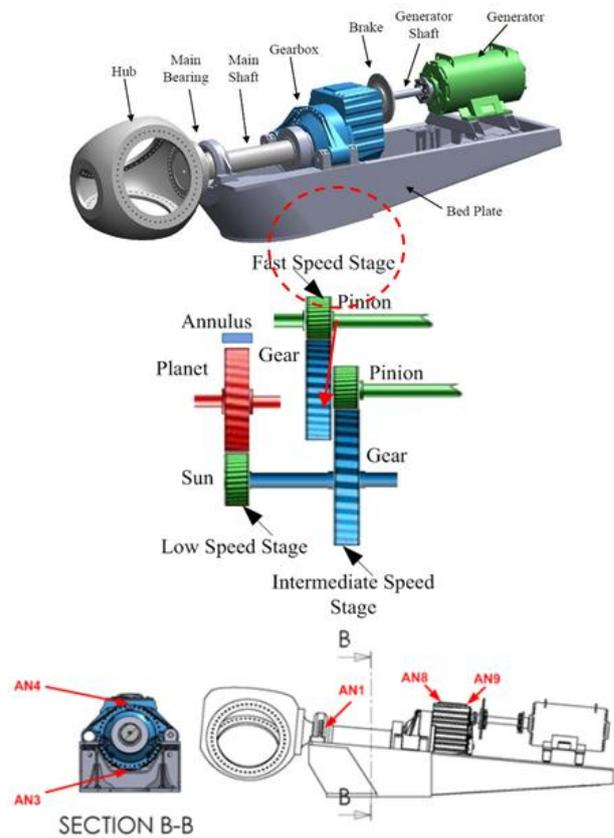
Figure 4. (a) GRC Drive train configuration (b) Planetary gearbox (c) Sensor locations. (courtesy of national renewable energy laboratory)
