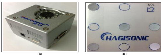
Figure 1. (a) The IR Sensor, (b) Passive Landmark
